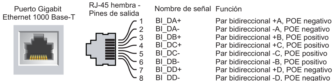
Figura 5 Pines del puerto Gigabit Ethernet
